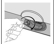
NOTE: Box must be closed and handle in horizontal position in order to lock box and remove key.
